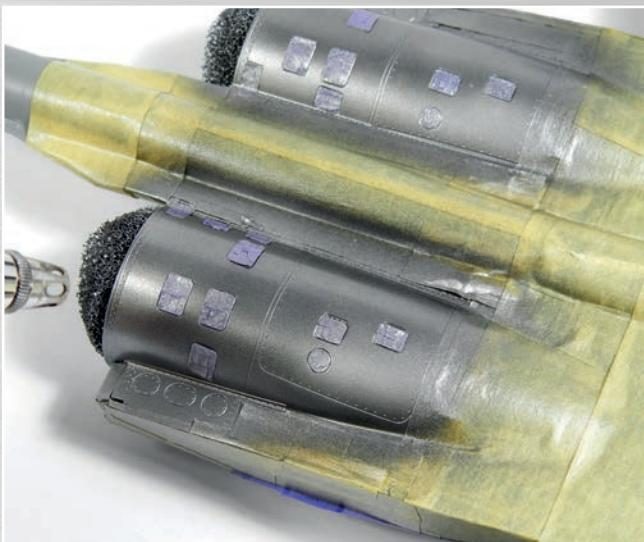
The transparent **A-Stand** colours are also perfect for replicating the iridescent effects on the nozzles and panels exposed to the extreme heat of jet aircraft's engines. First, apply the **A-Stand** metallic colours.
