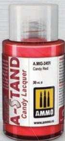
Use any **A-Stand** Candy colour you want, in this case it's Candy Red A.MIG-2451. Apply it in thin layers diluted with 50 % **A-Stand** Airbrush Thinner & Cleaner A.MIG-2013 so that you can avoid completely covering the silver colour. For a high gloss finish, apply a thick final layer sprayed at low pressure of about 1 or 1.2 bar (14-17psi), leaving a wet surface without flooding it.
