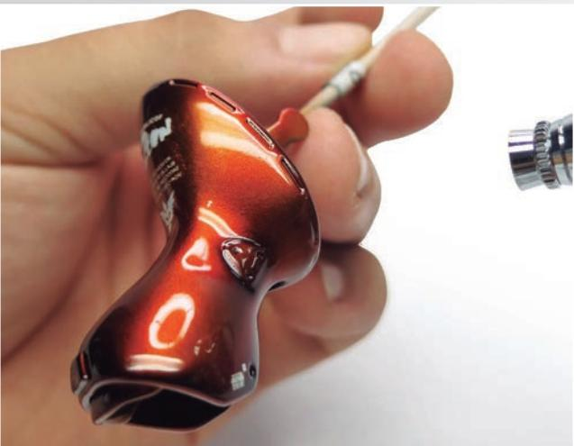
If you want to achieve a highly glossy surface on the decals, apply the transparent lacquer Transparent Medium A.MIG-2400 in the same way, using low pressure of about 1 or 1.2 bar (14-17 psi), leaving a wet surface without flooding it. Then allow the surface to dry 24 hours with the pieces covered.
