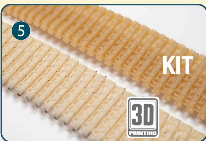
2. Little by little, remove the printing supports that are not need until the part is ready to assemble.
