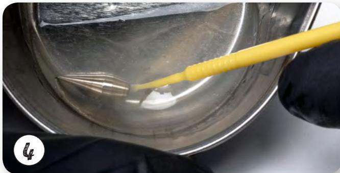
Again, dip the nozzle in the cleaner and rinse away any paint deposits with the help of a sniper brush.
